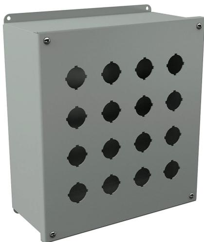
Wiegmann pushbutton enclosure, 16 holes, 30mm, NEMA 12, 12 x 11 x 5in (HxWxD), wall mount, carbon steel, ANSI 61 gray, powder coat finish, screw cover.
