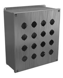
Wiegmann pushbutton enclosure, 16 holes, 30mm, NEMA 4/4X/12/13,  $12 \times 11 \times 5$  in (HxWxD), wall mount, 304 stainless steel, No. 3 intermediate polished finish, screw cover.
