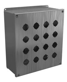
Wiegmann pushbutton enclosure, 16 holes, 30mm, NEMA 4/4X/12/13, 12 x 11 x 5in (HxWxD), wall mount, 304 stainless steel, No. 3 intermediate polished finish, screw cover.
