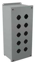
Wiegmann pushbutton enclosure, 10 holes, 30mm, NEMA 4/12/13, 14 x 6 x 5in (HxWxD), wall mount, carbon steel, ANSI 61 gray, powder coat finish, screw cover.
