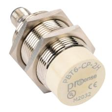
ProSense inductive proximity sensor, tubular, 30mm diameter x 60.3mm body, nickel-plated brass housing, PNP, N.C. output, 15mm sensing distance, non-flush, 300 Hz switching frequency, IP67, 4-pin M12 quick-disconnect.
