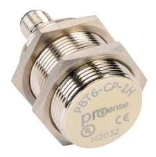
ProSense inductive proximity sensor, tubular, 30mm diameter x 60.3mm body, nickel-plated brass housing, PNP, N.C. output, 10mm sensing distance, flush, 300 Hz switching frequency, IP67, 4-pin M12 quick-disconnect.
