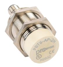
ProSense inductive proximity sensor, tubular, 30mm diameter x 56.6mm body, nickel-plated brass housing, PNP, N.O. output, 15mm sensing distance, non-flush, 300 Hz switching frequency, IP67, 4-pin M12 quick-disconnect.
