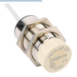
ProSense inductive proximity sensor, tubular, 30mm diameter x 49.2mm body, nickel-plated brass housing, PNP, N.O. output, 15mm sensing distance, non-flush, 300 Hz switching frequency, IP67, pigtail.
