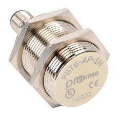
ProSense inductive proximity sensor, tubular, 30mm diameter x 56.6mm body, nickel-plated brass housing, PNP, N.O. output, 10mm sensing distance, flush, 300 Hz switching frequency, IP67, 4-pin M12 quick-disconnect.
