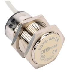
ProSense inductive proximity sensor, tubular, 30mm diameter x 49.2mm body, nickel-plated brass housing, PNP, N.O. output, 10mm sensing distance, flush, 300 Hz switching frequency, IP67, pigtail.
