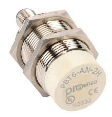
ProSense inductive proximity sensor, tubular, 30mm diameter x 67.7mm body, nickel-plated brass housing, NPN, N.O. output, 15mm sensing distance, non-flush, 300 Hz switching frequency, IP67, 4-pin M12 quick-disconnect.
