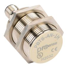
ProSense inductive proximity sensor, tubular, 30mm diameter x 67.7mm body, nickel-plated brass housing, NPN, N.O. output, 10mm sensing distance, flush, 300 Hz switching frequency, IP67, 4-pin M12 quick-disconnect.
