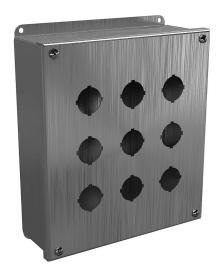
Wiegmann pushbutton enclosure, 9 holes, 30mm, NEMA 4/4X/12/13, 10 x 9 x 3in (HxWxD), wall mount, 304 stainless steel, No. 3 intermediate polished finish, screw cover.
