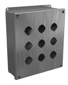
Wiegmann pushbutton enclosure, 9 holes, 30mm, NEMA 4/4X/12/13,  $10 \times 9 \times 3$  in (HxWxD), wall mount, 316L stainless steel, No. 3 intermediate polished finish, screw cover.
