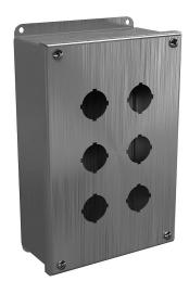
Wiegmann pushbutton enclosure, 6 holes, 30mm, NEMA 4/4X/12/13,  $10 \times 6 \times 3$  in (HxWxD), wall mount, 316L stainless steel, No. 3 intermediate polished finish, screw cover.
