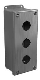
Wiegmann pushbutton enclosure, 3 holes, 30mm, NEMA 4/4X/12/13, 8 x 3 x 3in (HxWxD), wall mount, 304 stainless steel, No. 3 intermediate polished finish, screw cover.
