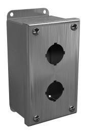
Wiegmann pushbutton enclosure, 2 holes, 30mm, NEMA 4/4X/12/13, 6 x 3 x 3in (HxWxD), wall mount, 316L stainless steel, No. 3 intermediate polished finish, screw cover.
