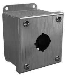
Wiegmann pushbutton enclosure, 1 hole, 30mm, NEMA 4/4X/12/13, 4 x 3 x 3in (HxWxD), wall mount, 304 stainless steel, No. 3 intermediate polished finish, screw cover.
