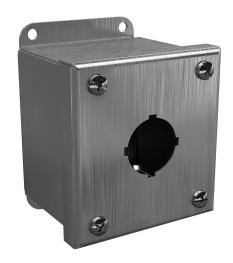
Wiegmann pushbutton enclosure, 1 hole, 30mm, NEMA 4/4X/12/13,  $4 \times 3 \times 3$  in (HxWxD), wall mount, 304 stainless steel, No. 3 intermediate polished finish, screw cover.
