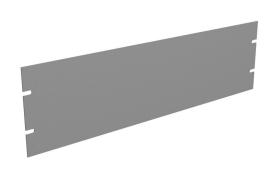
Hammond rack panel, 3U, 19in rack width, carbon steel, RAL 7035 light gray, powder coat finish.
