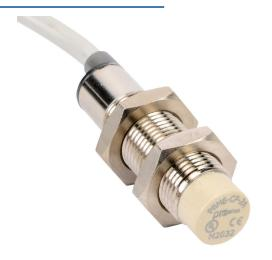
ProSense inductive proximity sensor, tubular, 12mm diameter x 48mm body, nickel-plated brass housing, PNP, N.C. output, 4mm sensing distance, non-flush, 1000 Hz switching frequency, IP67, pigtail.
