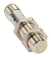
ProSense inductive proximity sensor, tubular, 12mm diameter x 48.4mm body, nickel-plated brass housing, PNP, N.C. output, 2mm sensing distance, flush, 1000 Hz switching frequency, IP67, 4-pin M12 quick-disconnect.
