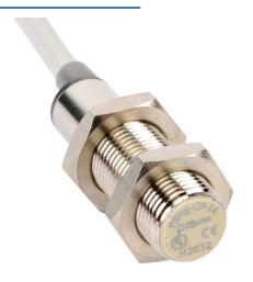
ProSense inductive proximity sensor, tubular, 12mm diameter x 42.5mm body, nickel-plated brass housing, PNP, N.C. output, 2mm sensing distance, flush, 1000 Hz switching frequency, IP67, pigtail.
