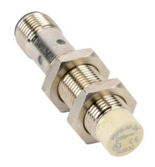
ProSense inductive proximity sensor, tubular, 12mm diameter x 53.9mm body, nickel-plated brass housing, PNP, N.O. output, 4mm sensing distance, non-flush, 1000 Hz switching frequency, IP67, 4-pin M12 quick-disconnect.
