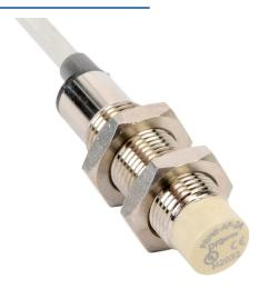
ProSense inductive proximity sensor, tubular, 12mm diameter x 48mm body, nickel-plated brass housing, PNP, N.O. output, 4mm sensing distance, non-flush, 1000 Hz switching frequency, IP67, pigtail.
