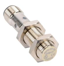
ProSense inductive proximity sensor, tubular, 12mm diameter x 48.4mm body, nickel-plated brass housing, PNP, N.O. output, 2mm sensing distance, flush, 1000 Hz switching frequency, IP67, 4-pin M12 quick-disconnect.
