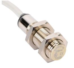
ProSense inductive proximity sensor, tubular, 12mm diameter x 42.5mm body, nickel-plated brass housing, PNP, N.O. output, 2mm sensing distance, flush, 1000 Hz switching frequency, IP67, pigtail.
