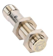
ProSense inductive proximity sensor, tubular, 12mm diameter x 48.4mm body, nickel-plated brass housing, NPN, N.O. output, 2mm sensing distance, flush, 1000 Hz switching frequency, IP67, 4-pin M12 quick-disconnect.
