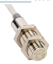
ProSense inductive proximity sensor, tubular, 12mm diameter x 42.5mm body, nickel-plated brass housing, NPN, N.O. output, 2mm sensing distance, flush, 1000 Hz switching frequency, IP67, pigtail.
