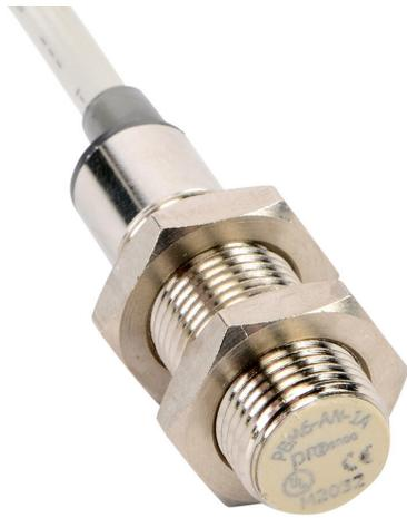
ProSense inductive proximity sensor, tubular, 12mm diameter x 42.5mm body, nickel-plated brass housing, NPN, N.O. output, 2mm sensing distance, flush, 1000 Hz switching frequency, IP67, pigtail.
