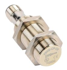
ProSense inductive proximity sensor, tubular, 18mm diameter x 46.9mm body, nickel-plated brass housing, PNP, N.C. output, 5mm sensing distance, flush, 1000 Hz switching frequency, IP67, 4-pin M12 quick-disconnect.
