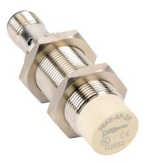
ProSense inductive proximity sensor, tubular, 18mm diameter x 65.2mm body, nickel-plated brass housing, PNP, N.O. output, 8mm sensing distance, non-flush, 1000 Hz switching frequency, IP67, 4-pin M12 quick-disconnect.
