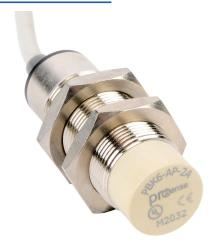
ProSense inductive proximity sensor, tubular, 18mm diameter x 55.7mm body, nickel-plated brass housing, PNP, N.O. output, 8mm sensing distance, non-flush, 1000 Hz switching frequency, IP67, pigtail.
