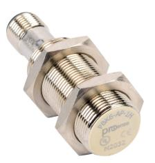
ProSense inductive proximity sensor, tubular, 18mm diameter x 56.4mm body, nickel-plated brass housing, PNP, N.O. output, 5mm sensing distance, flush, 1000 Hz switching frequency, IP67, 4-pin M12 quick-disconnect.
