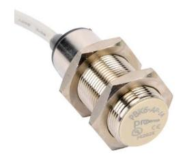
ProSense inductive proximity sensor, tubular, 18mm diameter x 46.9mm body, nickel-plated brass housing, PNP, N.O. output, 5mm sensing distance, flush, 1000 Hz switching frequency, IP67, pigtail.
