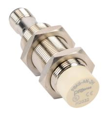
ProSense inductive proximity sensor, tubular, 18mm diameter x 65.2mm body, nickel-plated brass housing, NPN, N.O. output, 8mm sensing distance, non-flush, 1000 Hz switching frequency, IP67, 4-pin M12 quick-disconnect.
