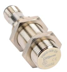
ProSense inductive proximity sensor, tubular, 18mm diameter x 56.4mm body, nickel-plated brass housing, NPN, N.O. output, 5mm sensing distance, flush, 1000 Hz switching frequency, IP67, 4-pin M12 quick-disconnect.
