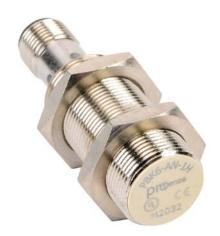
ProSense inductive proximity sensor, tubular, 18mm diameter x 56.4mm body, nickel-plated brass housing, NPN, N.O. output, 5mm sensing distance, flush, 1000 Hz switching frequency, IP67, 4-pin M12 quick-disconnect.
