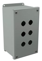
Wiegmann pushbutton enclosure, 6 holes, 22mm, NEMA 12/13, 9 x 5 x 4in (HxWxD), wall mount, carbon steel, ANSI 61 gray, powder coat finish, screw cover.
