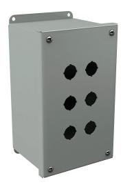
Wiegmann pushbutton enclosure, 6 holes, 22mm, NEMA 12/13, 9 x 5 x 4in (HxWxD), wall mount, carbon steel, ANSI 61 gray, powder coat finish, screw cover.
