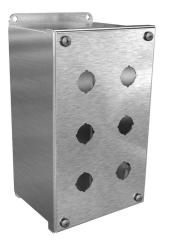
Wiegmann pushbutton enclosure, 6 holes, 22mm, NEMA 4/4X/12/13, 9 x 5 x 4in (HxWxD), wall mount, 304 stainless steel, No. 3 intermediate polished finish, screw cover.
