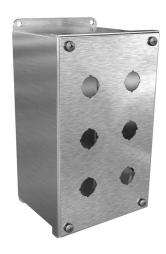
Wiegmann pushbutton enclosure, 6 holes, 22mm, NEMA 4/4X/12/13,  $9 \times 5 \times 4$  in (HxWxD), wall mount, 304 stainless steel, No. 3 intermediate polished finish, screw cover.
