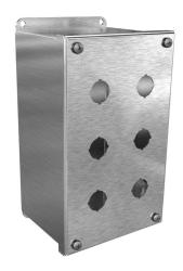
Wiegmann pushbutton enclosure, 6 holes, 22mm, NEMA 4/4X/12/13, 9 x 5 x 4in (HxWxD), wall mount, 316 stainless steel, No. 3 intermediate polished finish, screw cover.
