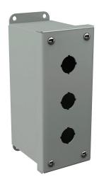
Wiegmann pushbutton enclosure, 3 holes, 22mm, NEMA 12/13, 7 x 3 x 4in (HxWxD), wall mount, carbon steel, ANSI 61 gray, powder coat finish, screw cover.
