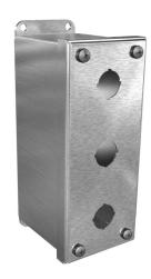
Wiegmann pushbutton enclosure, 3 holes, 22mm, NEMA 4/4X/12/13, 7 x 3 x 4in (HxWxD), wall mount, 316 stainless steel, No. 3 intermediate polished finish, screw cover.
