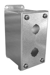
Wiegmann pushbutton enclosure, 2 holes, 22mm, NEMA 4/4X/12/13, 5 x 3 x 4in (HxWxD), wall mount, 304 stainless steel, No. 3 intermediate polished finish, screw cover.
