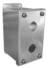
Wiegmann pushbutton enclosure, 2 holes, 22mm, NEMA 4/4X/12/13, 5 x 3 x 4in (HxWxD), wall mount, 316 stainless steel, No. 3 intermediate polished finish, screw cover.
