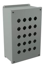
Wiegmann pushbutton enclosure, 20 holes, 22mm, NEMA 12/13, 13 x 8 x 5in (HxWxD), wall mount, carbon steel, ANSI 61 gray, powder coat finish, screw cover.
