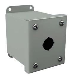
Wiegmann pushbutton enclosure, 1 hole, 22mm, NEMA 12/13, 3 x 3 x 4in (HxWxD), wall mount, carbon steel, ANSI 61 gray, powder coat finish, screw cover.
