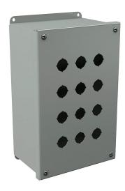
Wiegmann pushbutton enclosure, 12 holes, 22mm, NEMA 12/13, 10 x 7 x 4in (HxWxD), wall mount, carbon steel, ANSI 61 gray, powder coat finish, screw cover.
