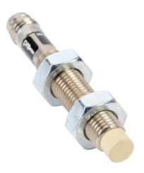
ProSense inductive proximity sensor, tubular, 8mm diameter x 53.9mm body, nickel-plated brass housing, PNP, N.C. output, 2mm sensing distance, non-flush, 1000 Hz switching frequency, IP67, 3-pin M8 quick-disconnect.
