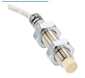
ProSense inductive proximity sensor, tubular, 8mm diameter x 44.4mm body, nickel-plated brass housing, PNP, N.C. output, 2mm sensing distance, non-flush, 1000 Hz switching frequency, IP67, pigtail.
