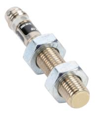
ProSense inductive proximity sensor, tubular, 8mm diameter x 49.9mm body, nickel-plated brass housing, PNP, N.C. output, 1.5mm sensing distance, flush, 1000 Hz switching frequency, IP67, 3-pin M8 quick-disconnect.
