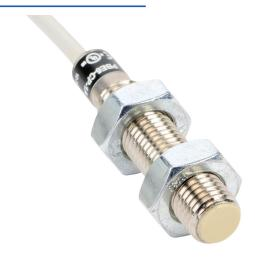
ProSense inductive proximity sensor, tubular, 8mm diameter x 40.4mm body, nickel-plated brass housing, PNP, N.C. output, 1.5mm sensing distance, flush, 1000 Hz switching frequency, IP67, pigtail.
