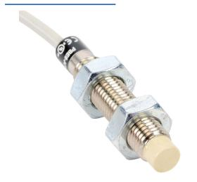
ProSense inductive proximity sensor, tubular, 8mm diameter x 44.4mm body, nickel-plated brass housing, PNP, N.O. output, 2mm sensing distance, non-flush, 1000 Hz switching frequency, IP67, pigtail.
