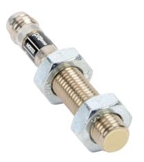
ProSense inductive proximity sensor, tubular, 8mm diameter x 49.9mm body, nickel-plated brass housing, PNP, N.O. output, 1.5mm sensing distance, flush, 1000 Hz switching frequency, IP67, 3-pin M8 quick-disconnect.
